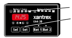
When the **FUNC** light is on, you can access Advanced Functions of the *Link 20*. The values for each function are changed using the **SET** and **SEL** keys.
