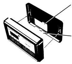
The phone cord to the *Freedom* inverter and the wires to the battery compartment may be led out the back of the nesting receptacle...
