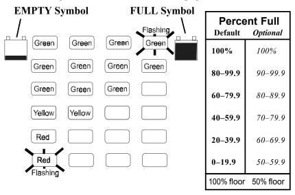
The Light Bars operate on *rate-corrected* amp hours. If you have heavily discharged a battery bank, the light bar may tell you to charge *before* you would normally make that decision based on the amp-hour display. See High Discharge Rates, page 26.
