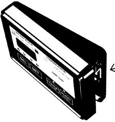
Press in on this tab with a thin metal coin while pulling one side of the unit away from the nesting receptacle.
