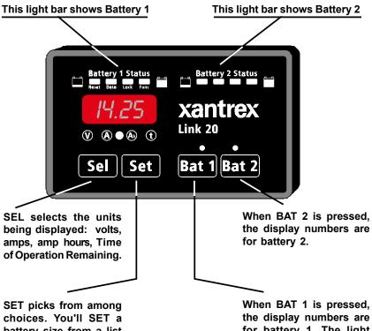
battery size from a list of choices when you first install your Link 20. the display numbers are for battery 1. The light above each button reminds you which battery you're looking at.
